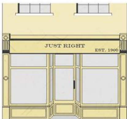
Figure 2: Example of traditional shopfront. The lettering is sympathetic in its font and size and in proportion to the depth of the fascia.
